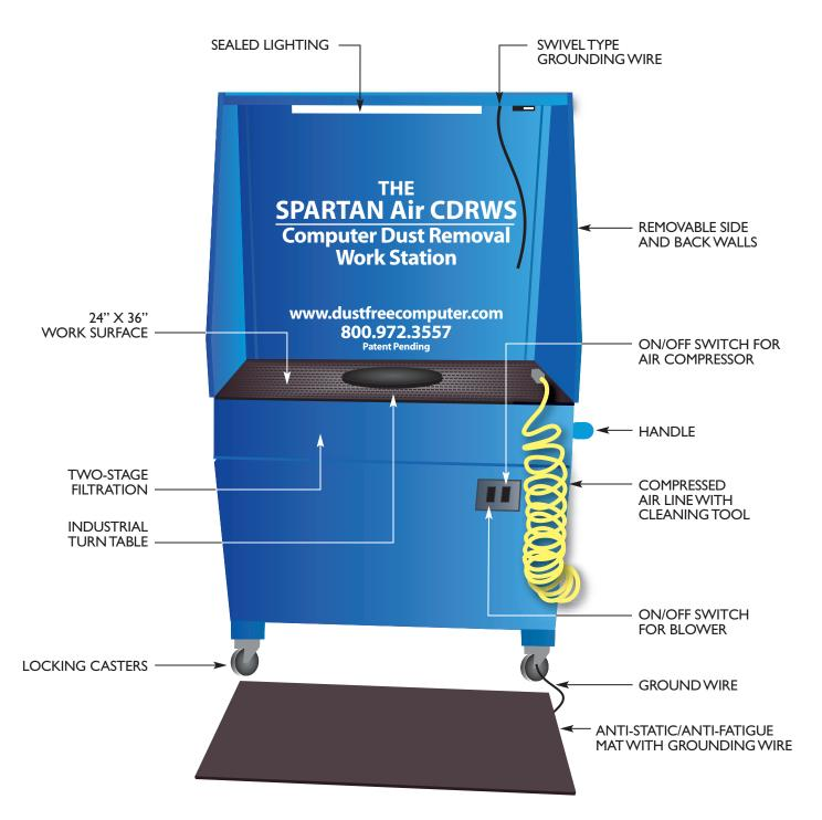
OVERALL DIMENSIONS: WITHOUT BACK/SIDE SHIELDS -38" H × 42"W × 27" D. WITH BACK/SIDE SHIELDS -70" H × 42"W × 27" D.
